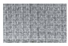
In comparison with TOPMESH 2, this laminate features an additional bonded layer between the filter mesh and the square weave support mesh. Constant low flow resistance and good backwashing capabilities enable higher pressure loads to be handled. TOPMESH 3 is particularly suitable for use with CIP (Cleaning In Place) filters.
