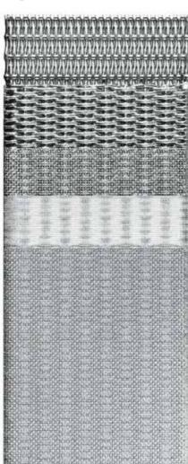
This lead-like filter medium consists of five different wire cloth layers, put together so precisely that they achieve the optimum combination of stability, filter fineness, flow rate and backwashing properties. POREMET is particularly suitable for fine and finest filtration applications at high pressures and harsh operating environments.
