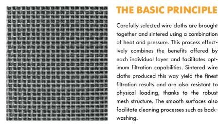
Carefully selected wire cloths are brought together and sintered using a combination of heat and pressure. This process effectively combines the benefits offered by each individual layer and facilitates optimum filtration capabilities. Sintered wire cloths produced this way yield the finest filtration results and are also resistant to physical loading, thanks to the robust mesh structure. The smooth surfaces also facilitate cleaning processes such as back-
